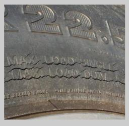
Gouge and cut in sidewall with cords exposed
